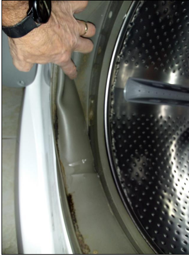
Mold growth at washer door seal
